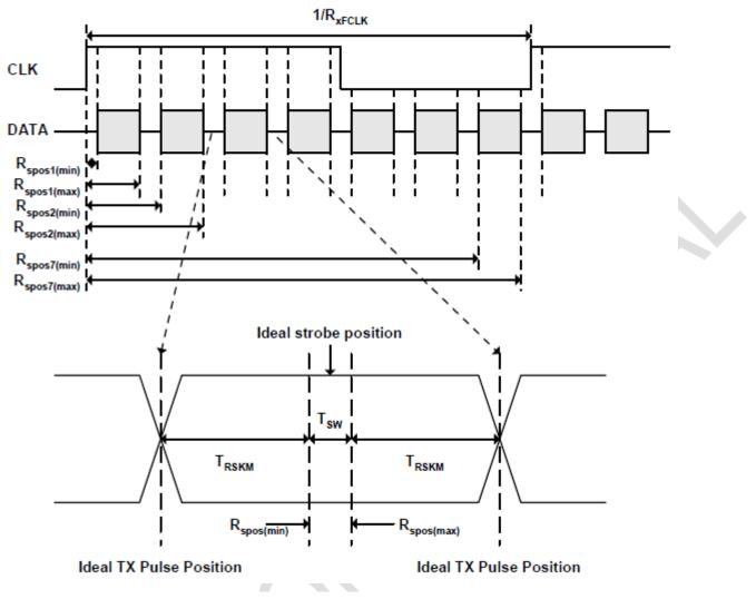
T<sub>RSKM</sub>: Receiver strobe margin R<sub>SPOS</sub>: Receiver strobe position
